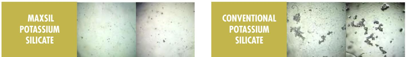
Figure 1: Visual difference of polymerization of potassium silicate of Maxsil vs. conventional potassium silicate diluted at 200ml/100L water and magnified at 60x under microscope
